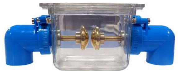
Fig. 1 : Vernier based Oil Test Cell
